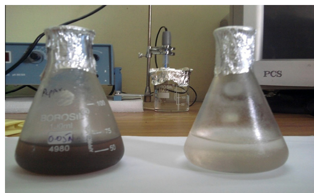
Figure 1 Aqueous solution of 0.001 M \text{AgNO}_3 with Pepper leaf extract.
